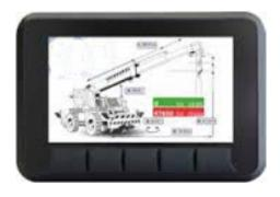
HVI204 is a 4" LCD Colour display with additional programmable keys available in the frame. This display is equipped with an ARM CORTEX processor, wich is programmable with a specific IDE environment available on request. HVI204 is including additional I/O ports for local data acquisition of hardware switches and sensors. The display area is QSVGA, with high contrast for good visibility under direct sunlight.
